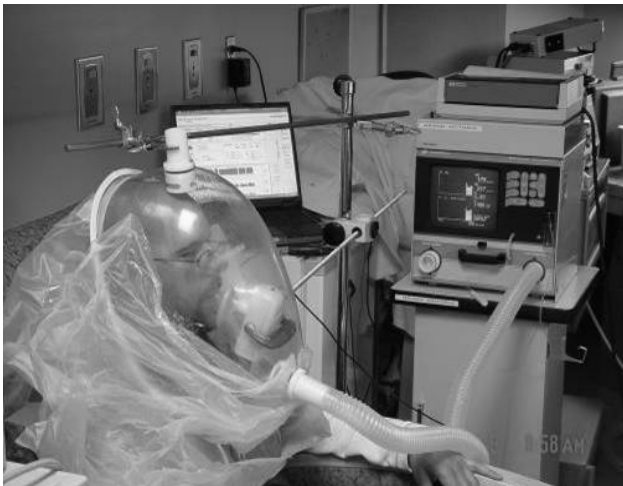
Figure 3. Photograph of a subject during simultaneous measurement with the DT & Gem (held by a C-clamp under the canopy) 19 .
